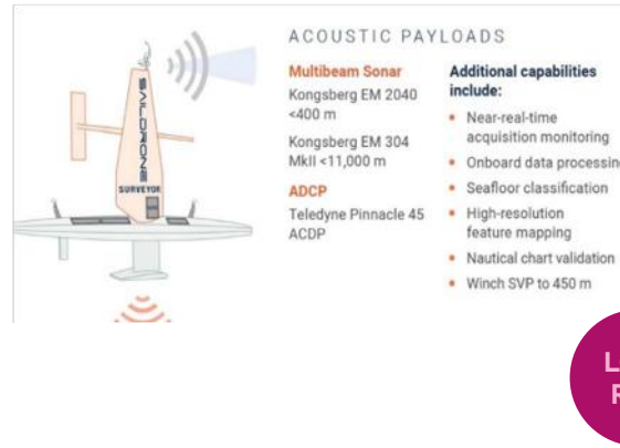
Figure 8. Photo of a SAILDRONE Surveyor, alongside with the technical specifications of its acoustic payloads as presented in March 2023 at SubOptic Conference in Bangkok, Thailand. Photo and graphic by SAILDRONE.
